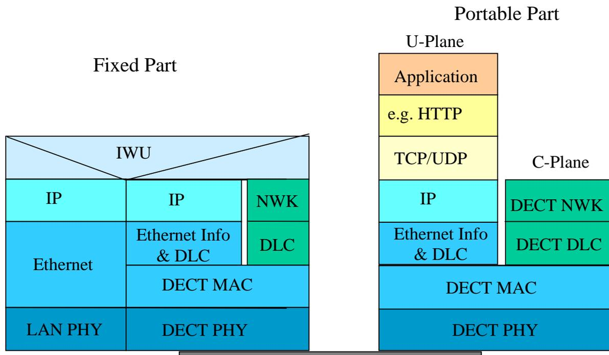
Figure 10: Protocol architecture for transport of IP-packets
