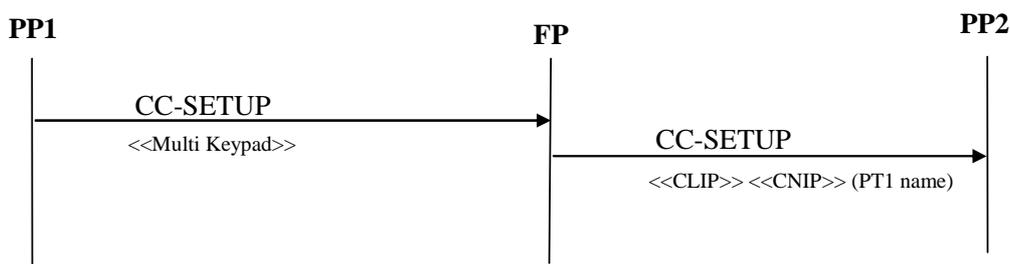
**Figure 78b: Internal call using <<CNIP>> from FP**
