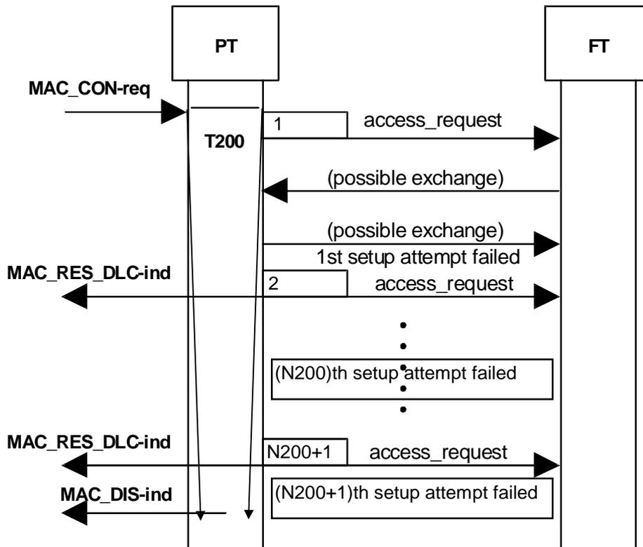
Figure 88: Bearer setup attempt fails N200+1 times
