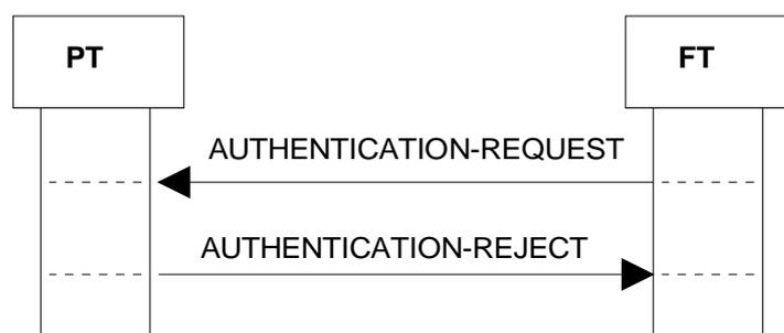
**Figure 51: Authentication algorithm/key not supported by the PT**
