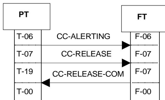
Figure 39: PT release the incoming call transaction
