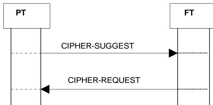
Figure 67: Ciphering, PT initiated
