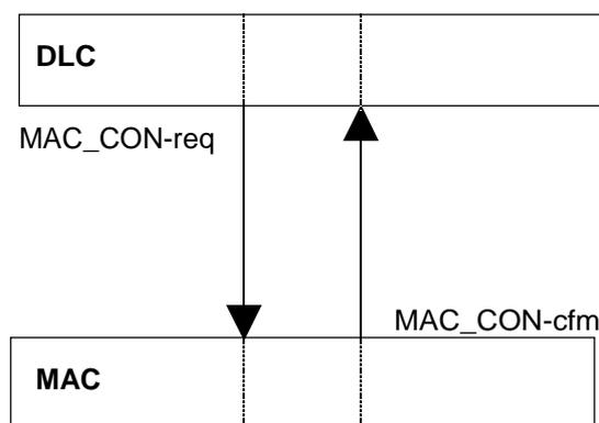
Figure 80: Establishment of a MAC connection initiating side
