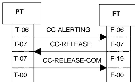
Figure 38: FT releases the incoming call transaction
