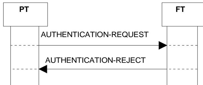
Figure 48: Authentication algorithm/key not supported by the FT
