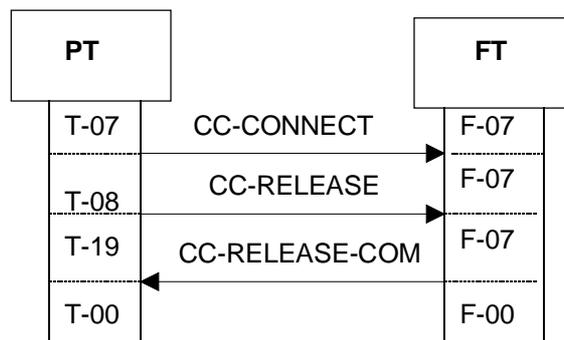
**Figure 43: PT releases the incoming call transaction**
