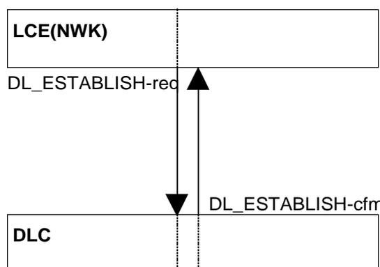
Figure 72: Direct PT initiated link establishment, initiating side
